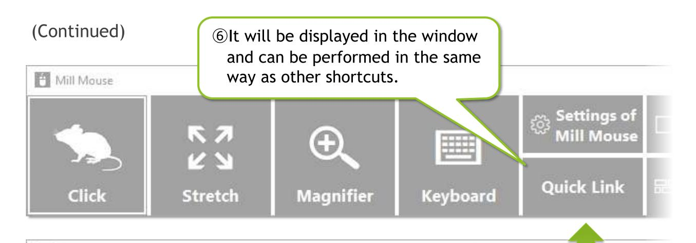
The state of the shortcut key will remain pressed and the button color will be reversed. If you press the button again, the keys will be released and the button color will be restored.
