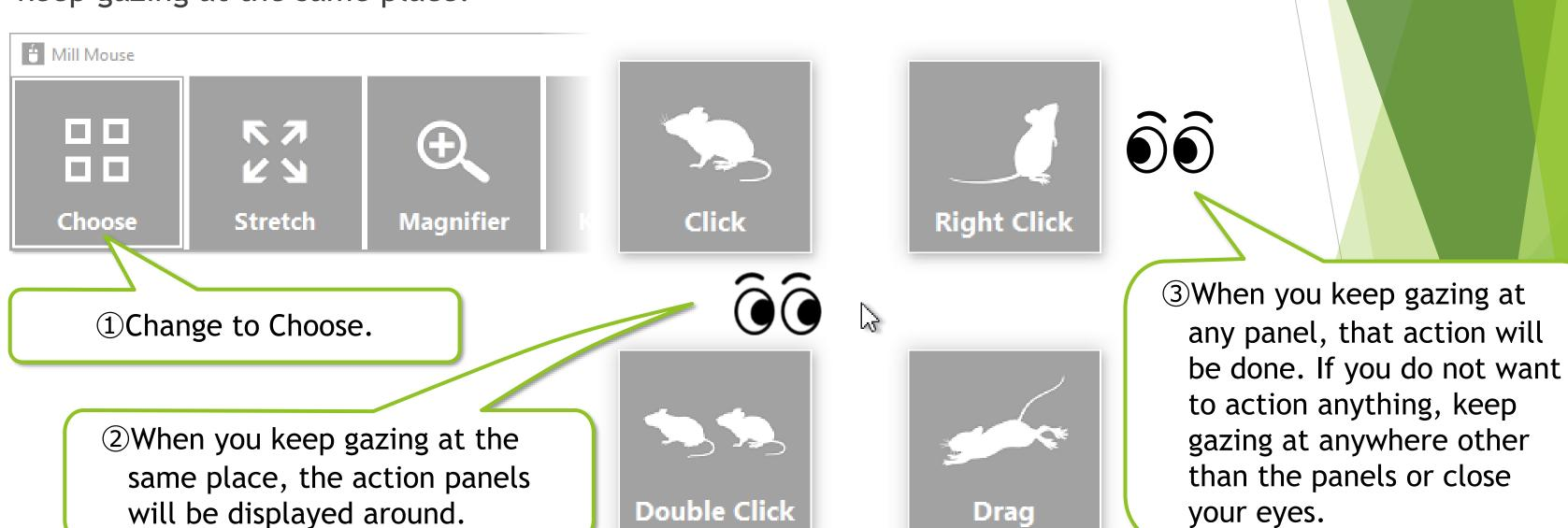
If you keep gazing on the touch keyboard or the on-screen keyboard, the click action will be done without displaying the action panels.
