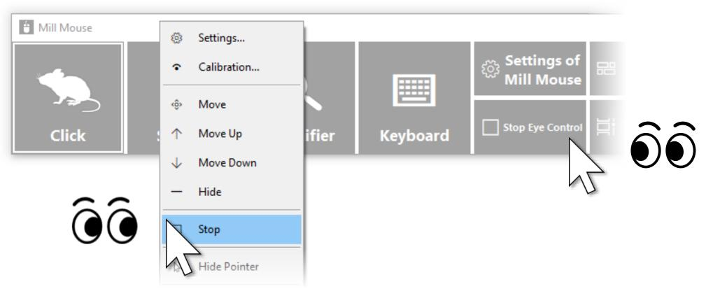
Unlike the physical mouse operation described above, the stop will not be canceled automatically. You can cancel the stop by looking at the upper left corner of the desktop screen and re-displaying the window.
