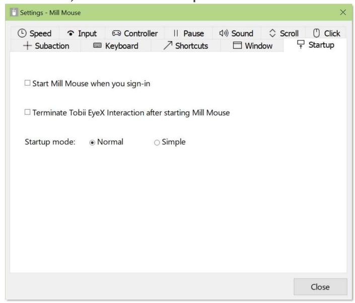
If you set the startup mode to Simple, Mill Mouse will run in simple mode. In simple mode, the available functions and display items are limited. It has the following differences from normal mode.
