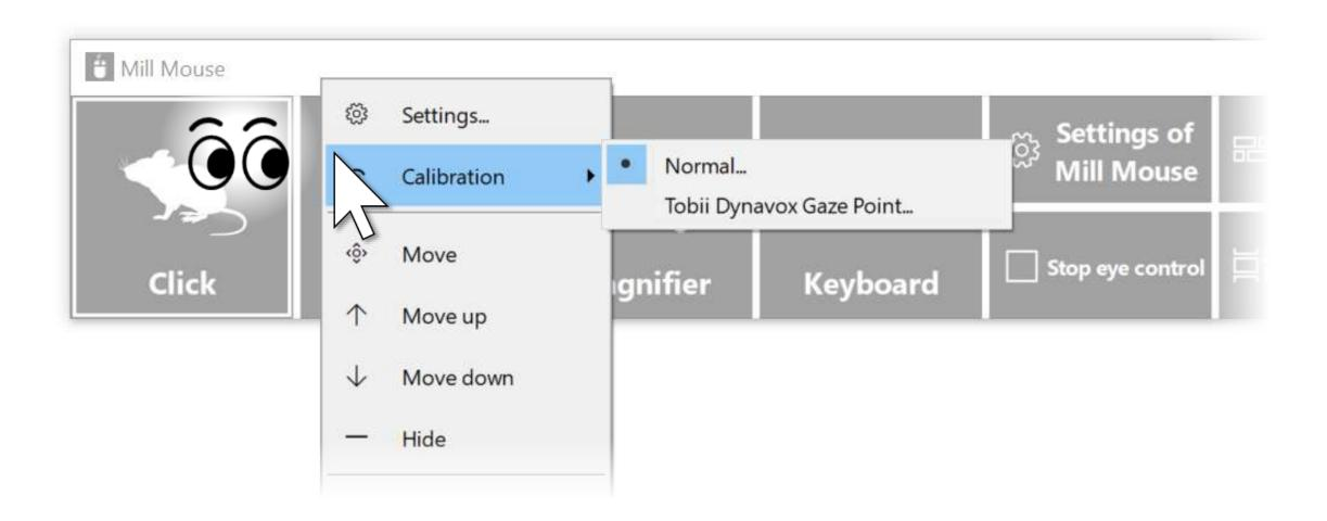
To customize the calibration settings of Tobii Dynavox Gaze Point, run Gaze Point Settings separately from Mill Mouse.
