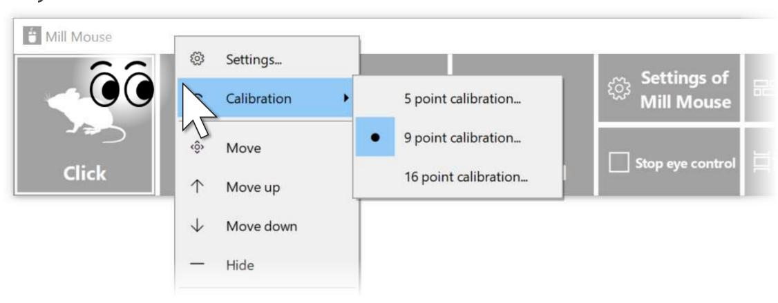
The greater the number of calibration points, the longer it takes to calibrate, but the more accurate the eye tracking will be.
