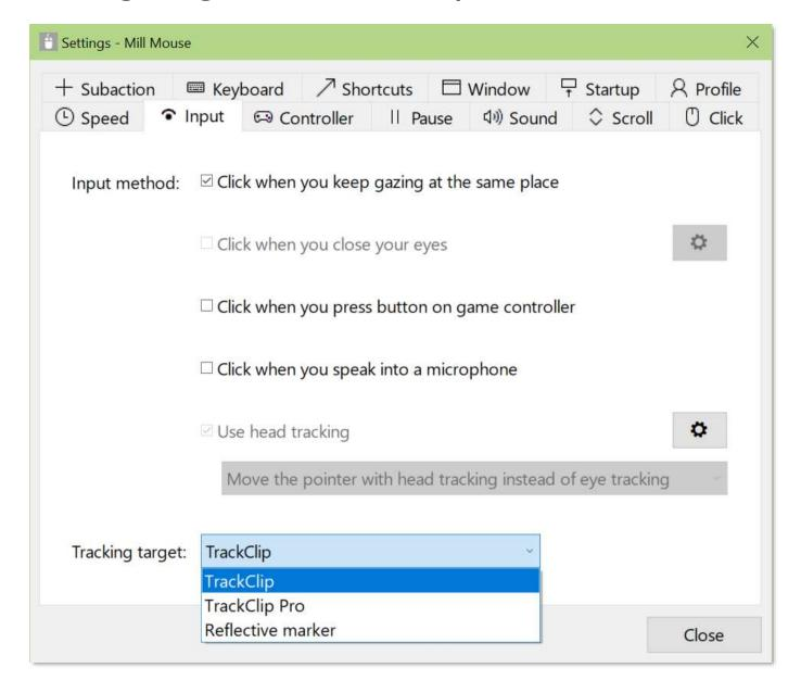
It can also be used with a commercial reflective material instead of TrackClip or TrackClip Pro. To use with a reflective material, change 'Tracking target' to 'Reflective marker'. You can move the mouse pointer by moving the reflective material up, down, left or right in front of the TrackIR 5 camera.
